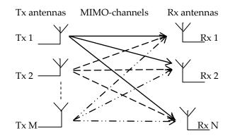
Figure 3 Block Diagram of a generic MIMO system with M transmitters and N receivers
