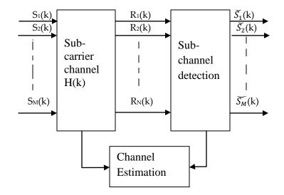
Figure 4: Baseband block diagram of k subcarrier channel in MIMO-OFDM system
