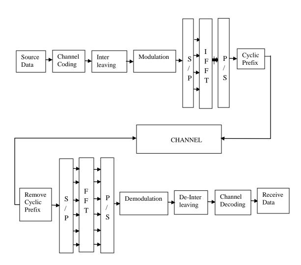
Figure 1: Block Diagram of OFDM system
